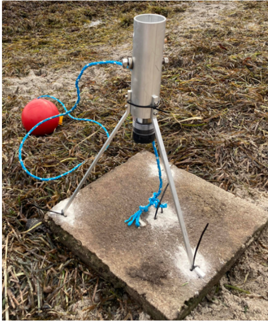
(a) Stand with miniDOT and 40 cm x 40 cm concrete tile used as base.
