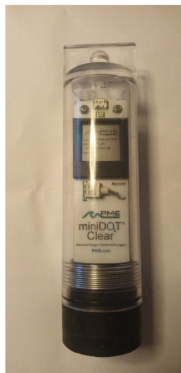
(a) The New oxygen logger (miniDOT) that is being used for the final oxygen method.
