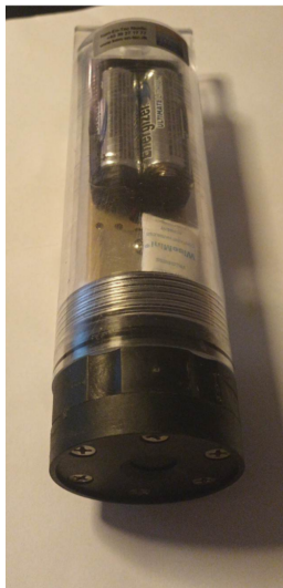
(a) The New oxygen logger (miniDOT) that is being used for the final oxygen method.
