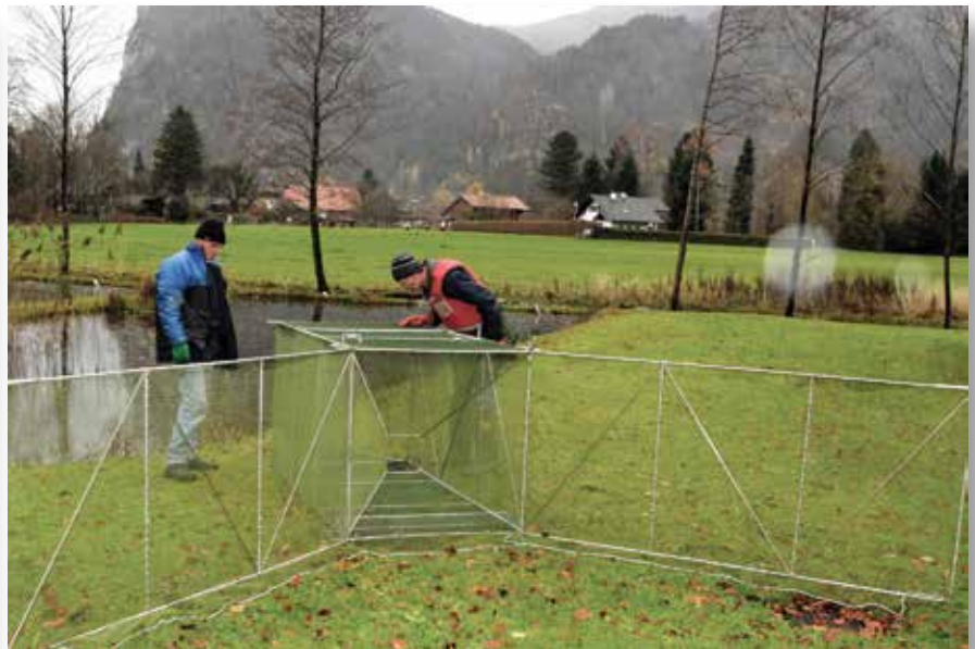
Figure 8.10 A fish trap showing outstretched mesh 'wings' that guide fishes in to a central holding compartment. Photo courtesy of W Hauer.
